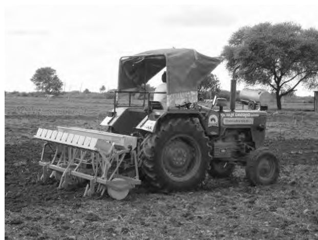
Plate 4. Field evaluation of Zero till planter for cotton in field
