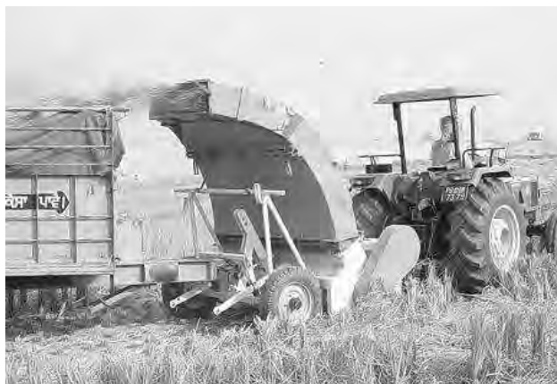
Plate 17. Flail type chopper cum loader
