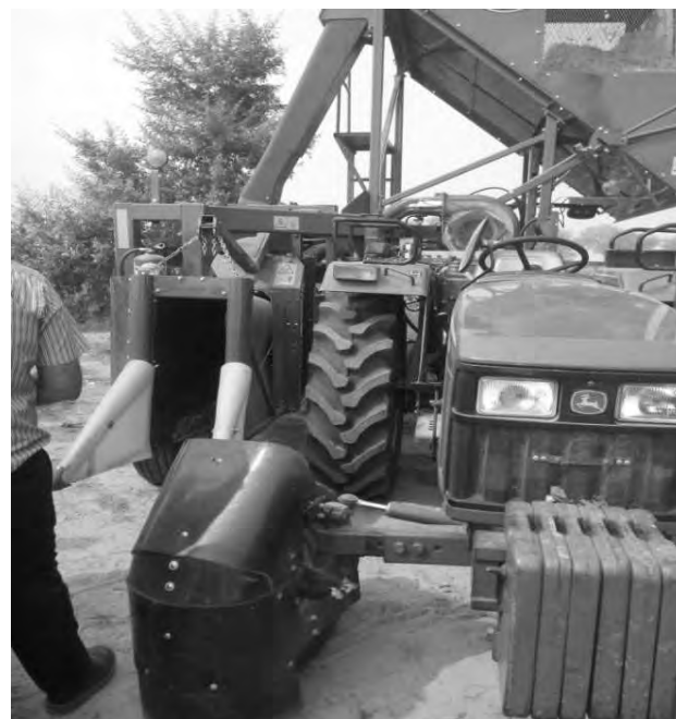
Fig. 2. Single row cotton picker attempted in India spindle type picker based mechanism appeared to be working satisfactorily for picking of cotton. This method was also evaluated in Indian cotton farms by cotton pickers imported from then USSR [14]. However, the further progress in this direction was constrained by the fall of former USSR.
