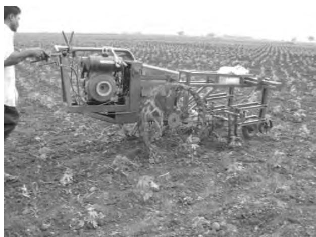
Plate 10. Self propelled inter row cultivator A self propelled inter row cultivator was
