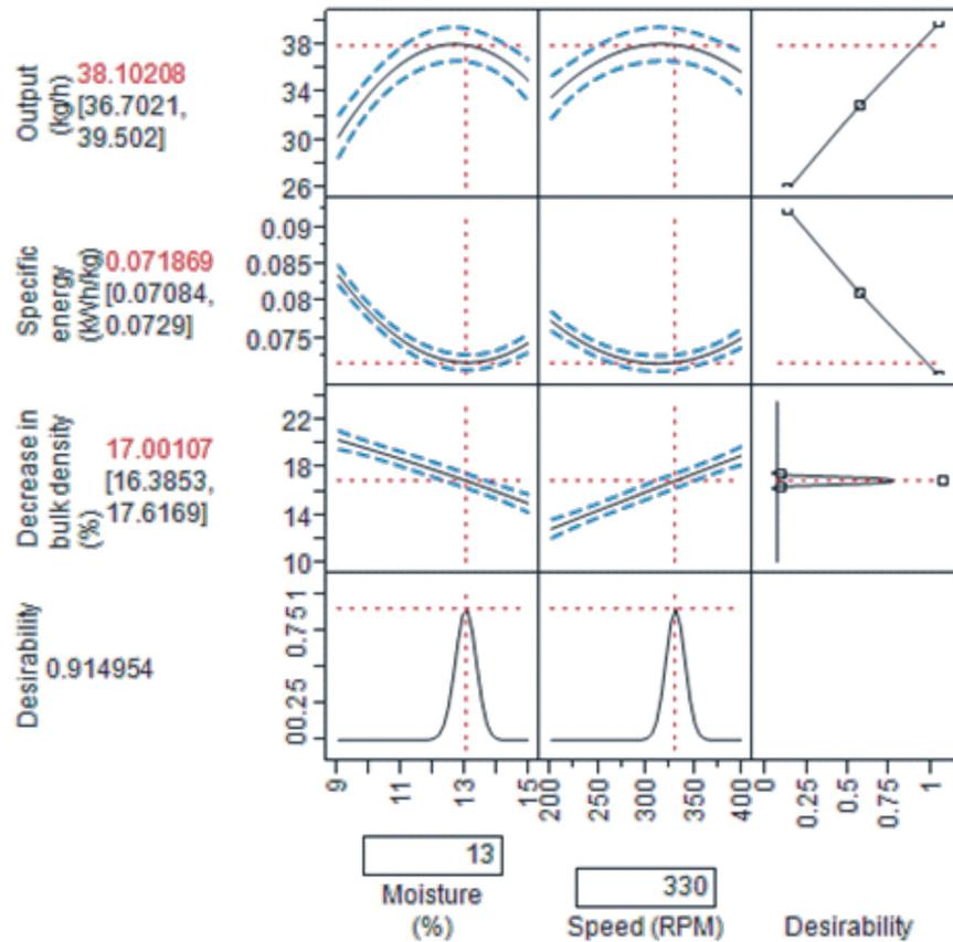
Fig.8. Desirability and levels of moisture and speed by multiple response optimisation for M3
