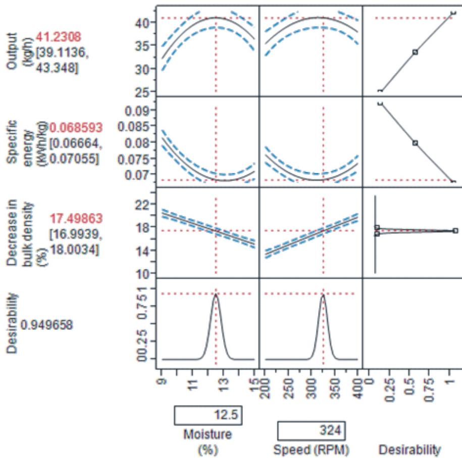
**Fig.6.** Desirability and levels of moisture and speed by multiple response optimisation for M1
