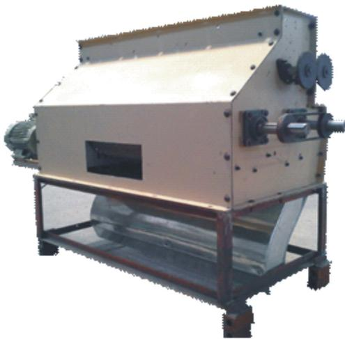
**Fig. 1.** Spike cylinder feeder (M1)
