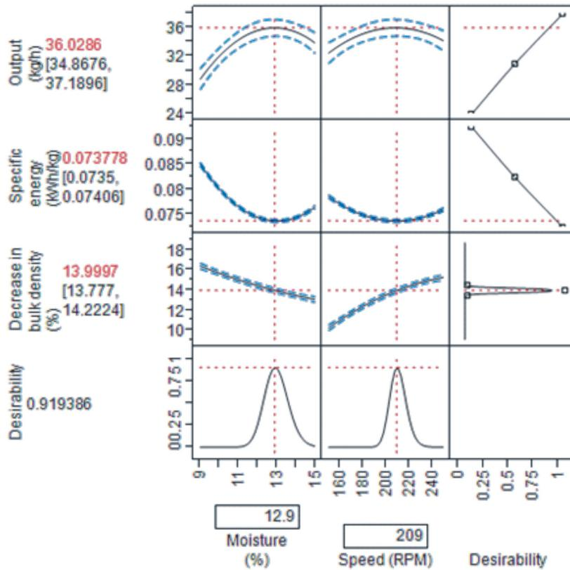
Fig.7. Desirability and levels of moisture and speed by multiple response optimisation for M2
